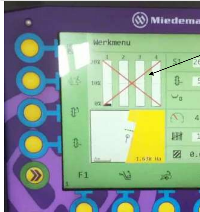
Picture 8: All rows have passed the headland line, the drive is switched off, the machine does not plant anymore
