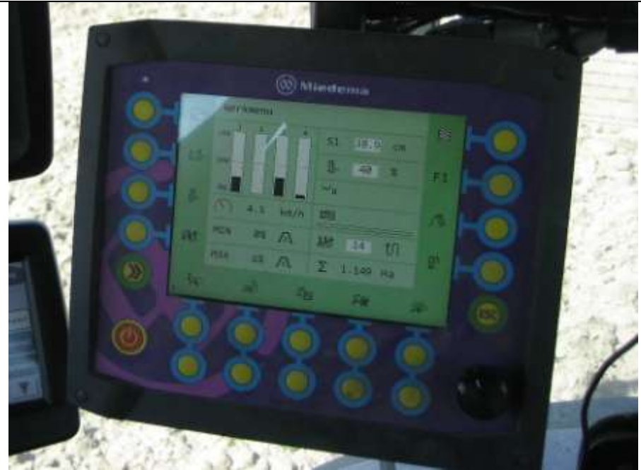
Picture 2: HMI control display to operate the planter
