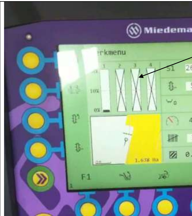
Picture 7: Row 4, 3 and 2 have passed the headland line, those 3 rows are switched off
